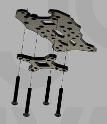
USE THE SPLIT PLATE TOP, THE X ISOLATION PLATE AND 4 X 25MM SCREWS TO SECURE BOTH PLATES.
