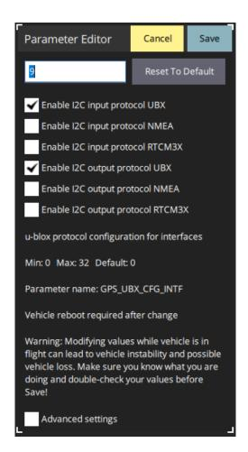
IMPORTANT! These options for GPS\_UBX\_CFG\_INTF must be enabled for the RID module to work properly! If your RID module LED is solid red, solid green, or not lit at all, double check that GPS\_UBX\_CFG\_INTF is configured properly.
