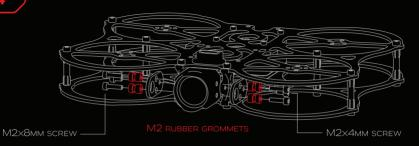
4. IN ORDER TO MOUNT THE DJI O3 CAMERA TO THE SIDE PLATES INSTALL THE M2 RUBBER GROMMETS INSIDE OF THE PLATES. USE M2x8mm SCREWS TO MOUNT THE CAMERA TO THE SIDE PLATES AND USE M2x4mm TO MOUNT THE CAMERA ASSEMBLY TO THE ALUMINUM MOUNTS
