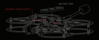
6. STICK THE BATTERY PAD TO THE TOP PLATE AND INSTALL THE STRAP INTO THE TOP PLATE SLOTS
