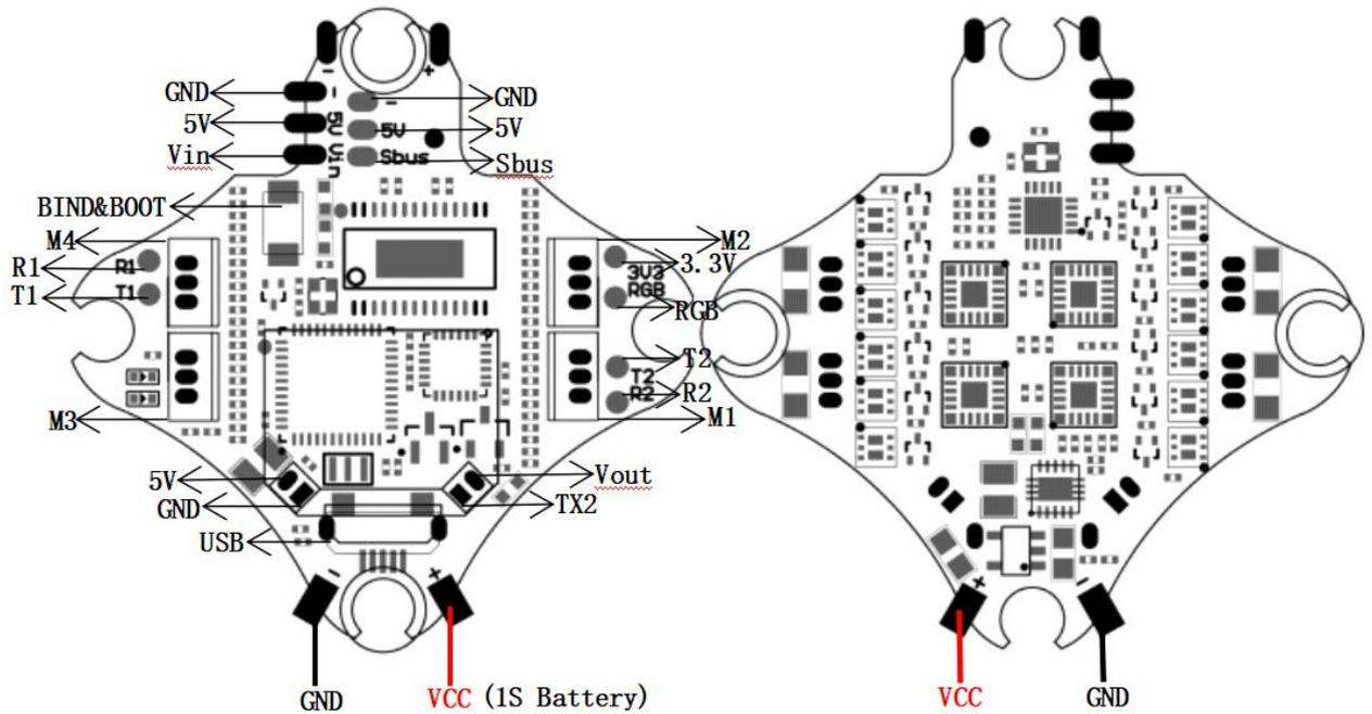
This flight controller has a MCU(STM32F411CEU6) with a MPU6000 gyro. Tinyhawk III flight controller comes pre-programmed and properly tuned for optimal flight. For a full tune and configuration setting file (CLI dump file) please visit <https://emax-usa.com/> for the CLI dump file.
