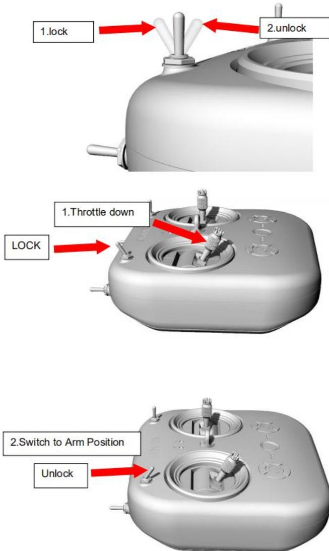
Arming refers to setting Tinyhawk III to begin flying. When Tinyhawk III is powered on for the first time, it will not spin the propeller until it is armed.
